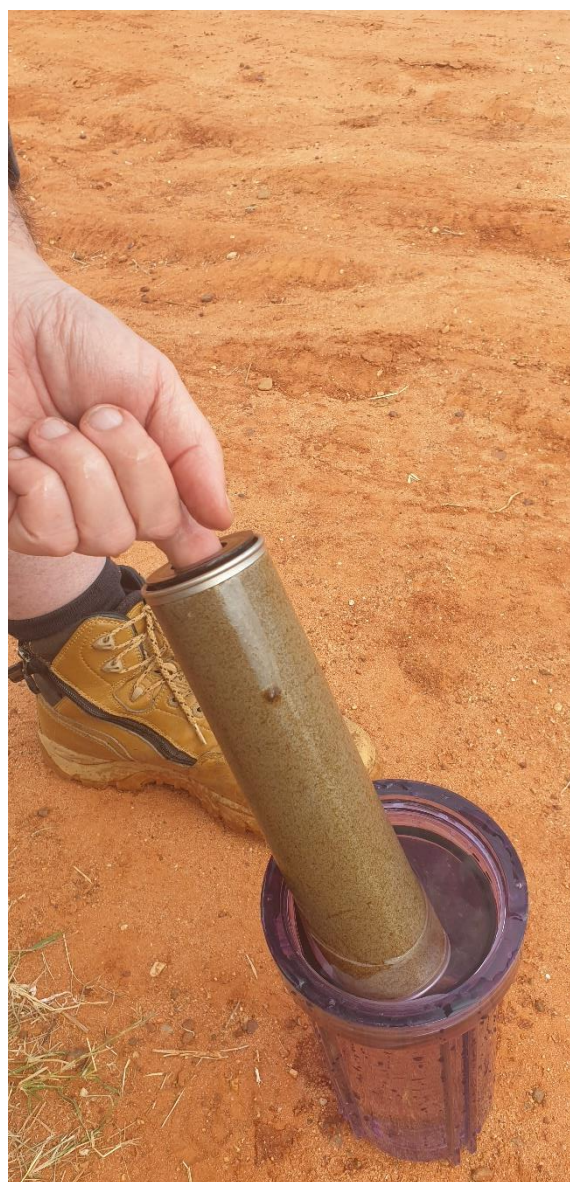
Figure 12 Inner particulate filtration unit displaying dirt and slime (photo credit: Trevor Harvey).
