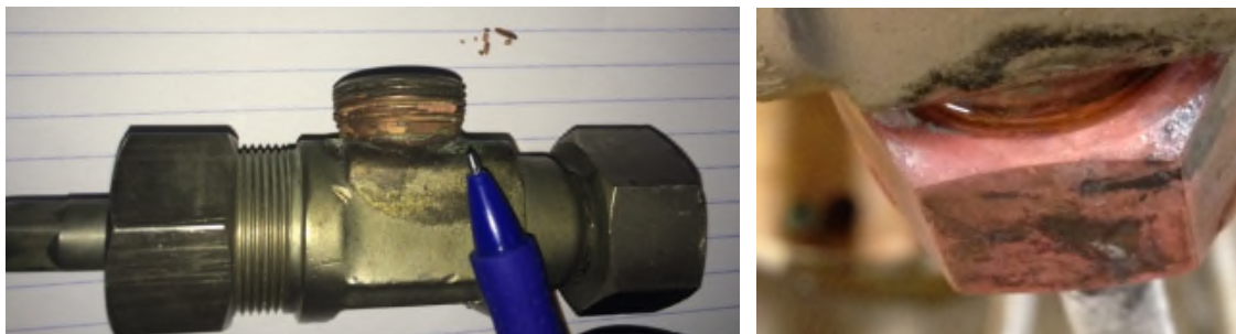
Figure 2: Brittle threads on valve (left), moisture in pigtail nut at Greenvale (right)
